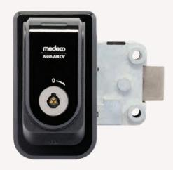
An LED provides visual feedback to the user on the current state of the lock. If the Lock PCB and XT Key are in agreement that access is granted, the Lock PCB will provide power to the internal motor/bolt blocker and the user is allowed to rotate the key to unlock the lock. If the XT Key is not authorized, the user will be prevented from unlocking the safe lock.
